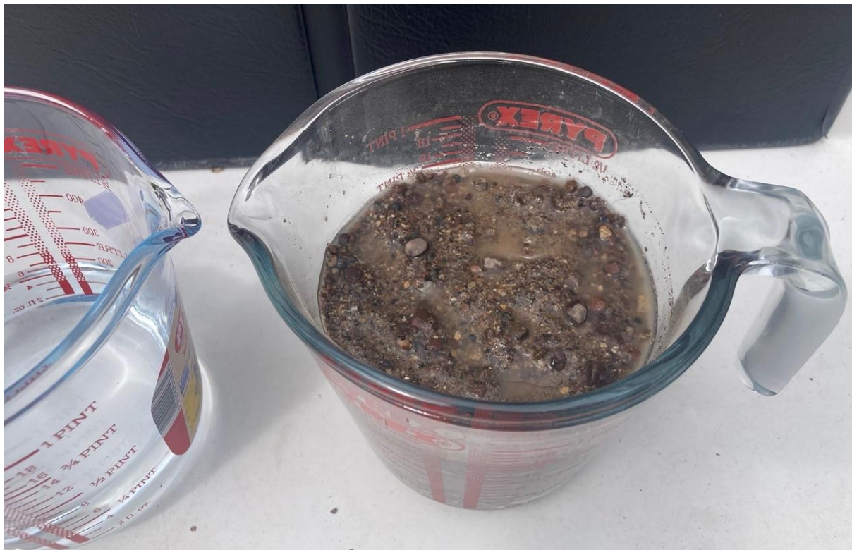
Plate 22: Water added to the aggregate container until it comes to the top of the aggregate at the 400ml mark.
