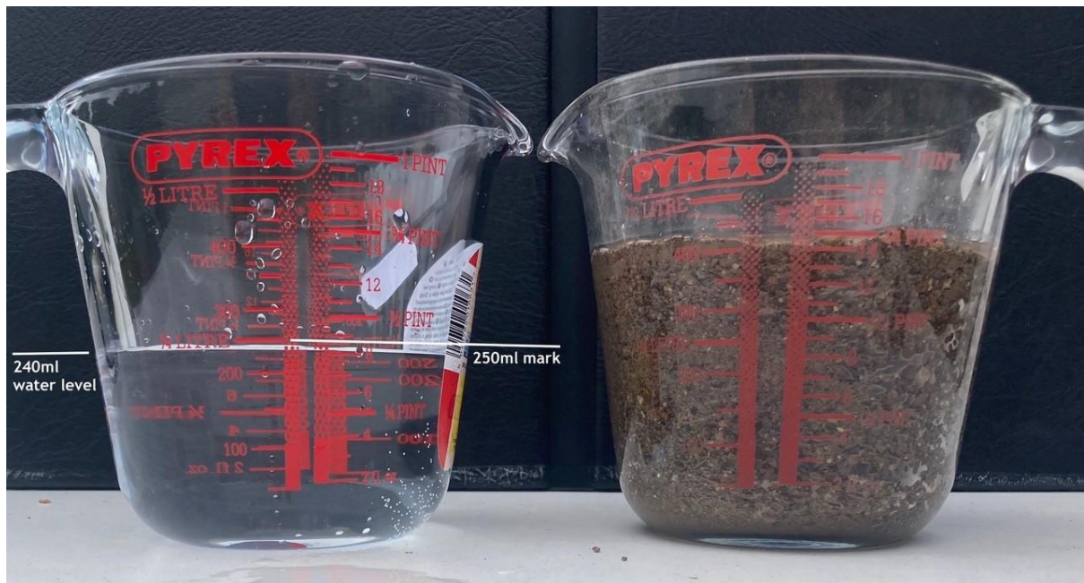
Plate 23: 240ml of water is left in the container, so 160ml was required to fill the voids in the aggregate. The lime to aggregate ratio for this selected aggregate is therefore 160:400 or 1:2.5. It will vary with other aggregate mixes.
