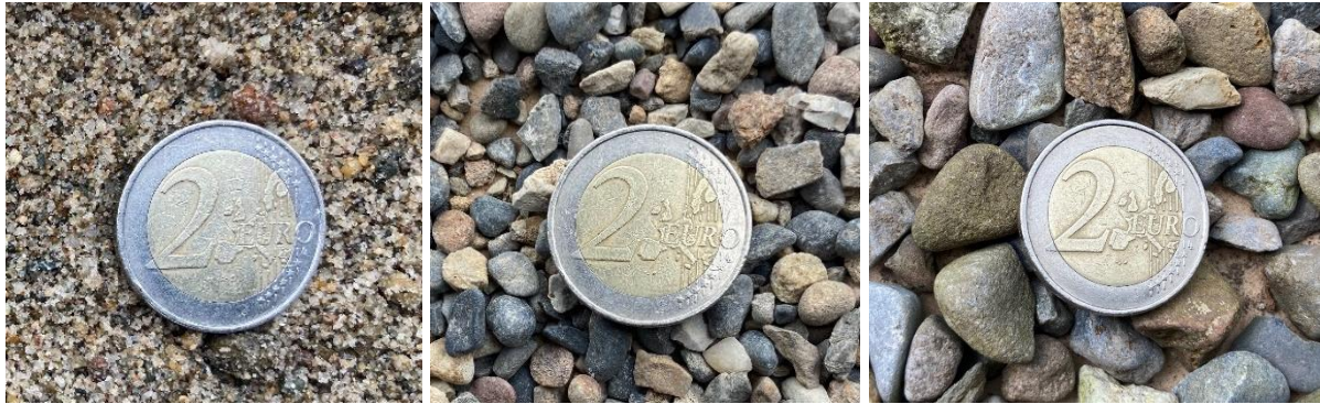
Plates 10–12: Sample sand 5mm and smaller (left), and samples of different grades of aggregate (centre and right) that can be combined to achieve the correct mortar mix depending on the requirements as determined from the sample area.
