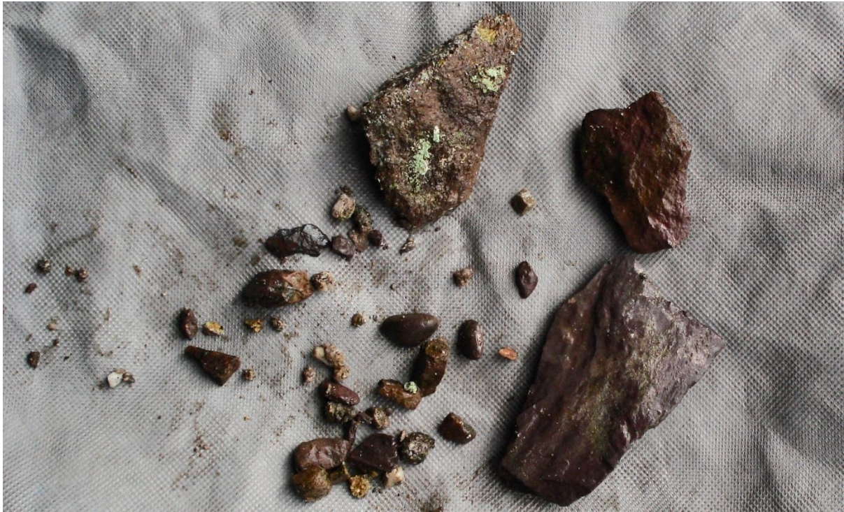
Plate 7: The same raked-out material washed for re-use in the repointing. The salvaged stones will help to decide the size of aggregate required in the mortar generally.
