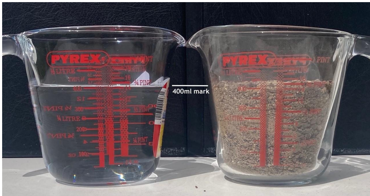
Plate 21: Two graduated containers filled to the 400ml mark, with water on the left, and dry aggregate mix on the right.
